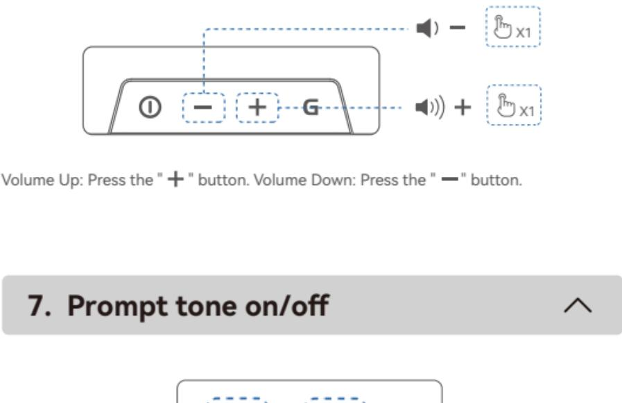
Power on: Press and hold the "①" button for 1s.
